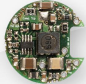
Holes for Connector Pins X1 to X6 have 0.8mm diameter
